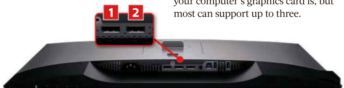
Link DisplayPort monitors using their DisplayPort In (1) and DisplayPort Out ports (2)
