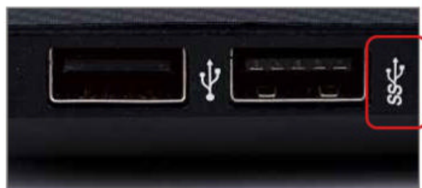
The 'SS' next to the port on the right indicates that it's USB 3.1 standard
