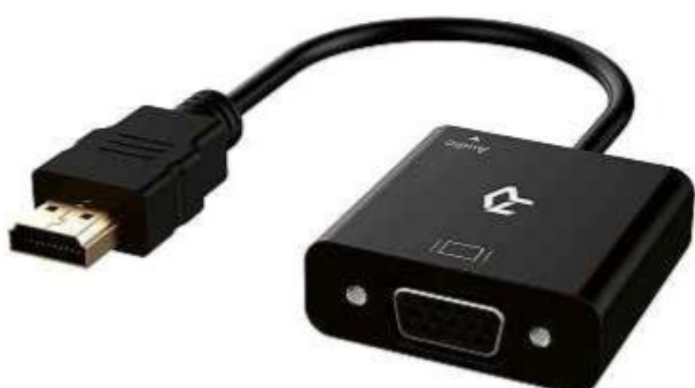
This HDMI-to-VGA adapter connects the audio output of an HDMI port to a set of speakers
