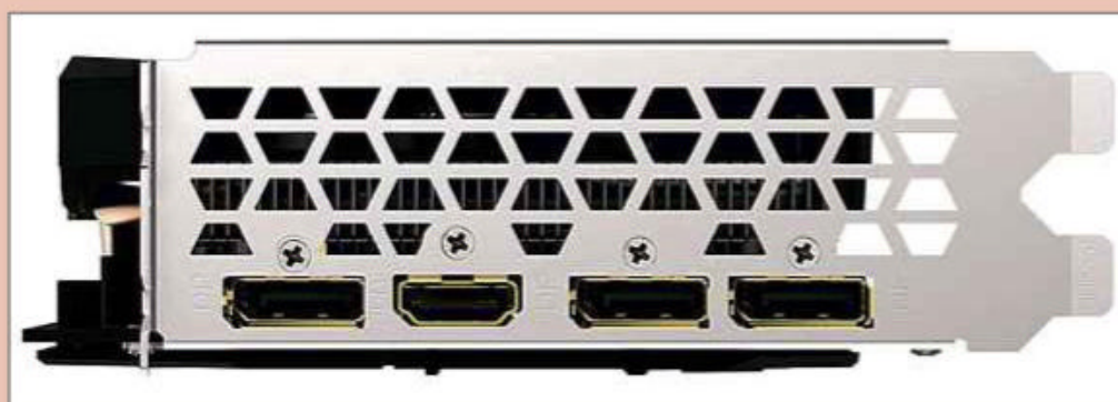
The Gigabyte GeForce GTX 1660 graphics card has one HDMI and three DisplayPort sockets
