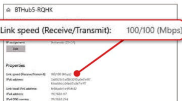
A link speed of 100/100 means your computer can transfer files only up to 100Mbps
